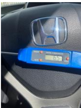
Temp Reading – Heaters on cold
